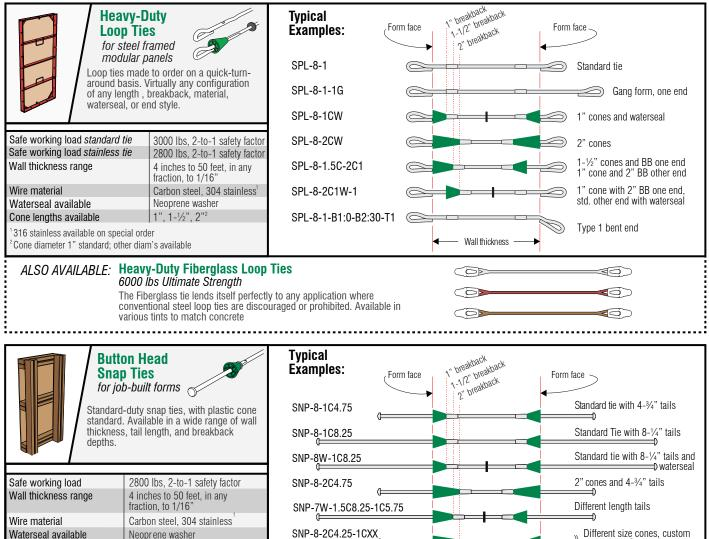
Waterseal availableNeoprene washerSNP-8-2C4.25Cone lengths available1", 1-½", 2"2Tail length1" minimum, to any length'316 stainless available on special order2 Cone diameter 1" standard; other diam's available
